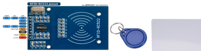
Figure 4. RC522 Reader and Tag
