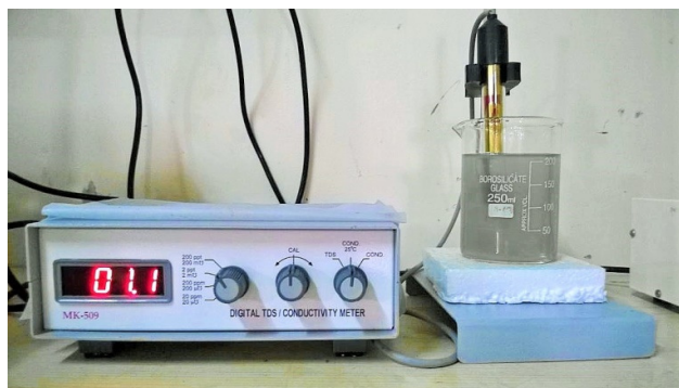
Fig23: electrical conductivity meter
