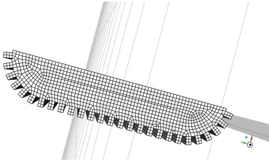
**Fig.1** Mesh geometry of heat pipe
