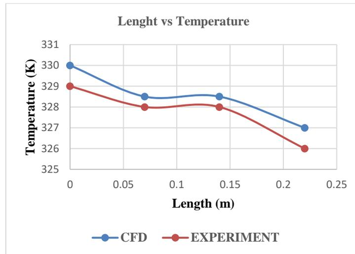
**Fig.5** Temperature variation along the heat pipe in CFD analysis and experimentation
