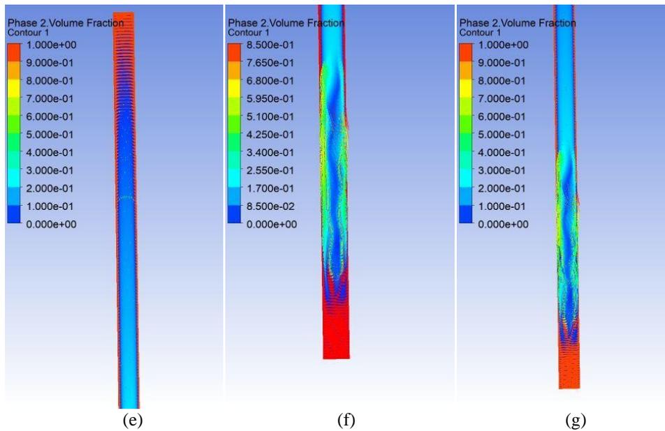
**Fig.3** Contours of volume fraction at different time steps when porosity is 42% at a heat input of 40W
