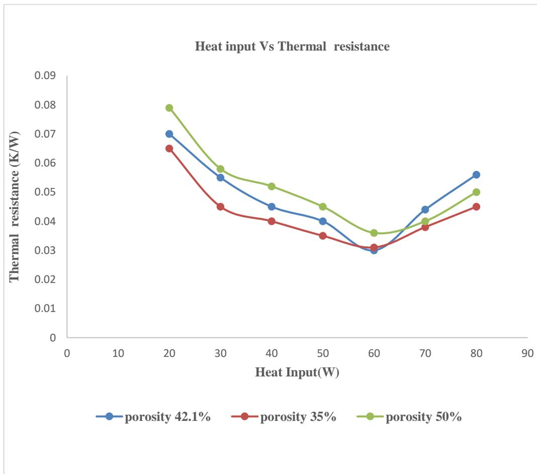
**Fig.6** Plot between the thermal resistance and heat input at different porosity values
