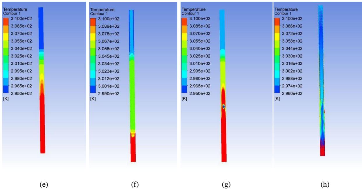
**Fig. 2** Temperature distribution along the heat pipe when porosity is 42% at a heat input of 40W
